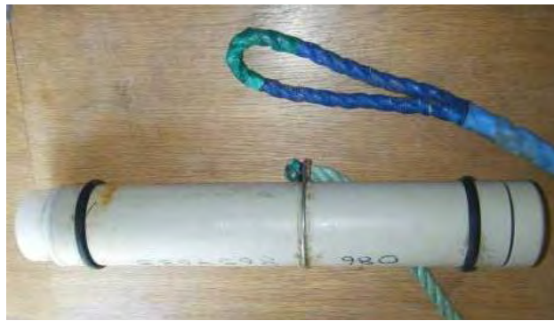
Figure 6.3 C-POD unit by Chelonia Ltd.
